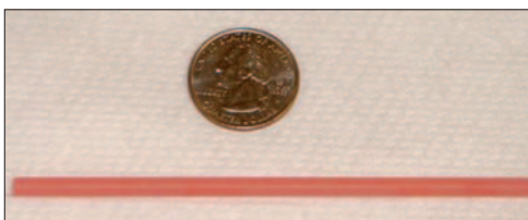
Fig. 19 A rod of Nd:YAG crystal active medium, compared to a coin to reflect the size
